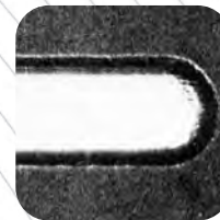
DURALLOY® TDC Layer thickness: 2.5µm
