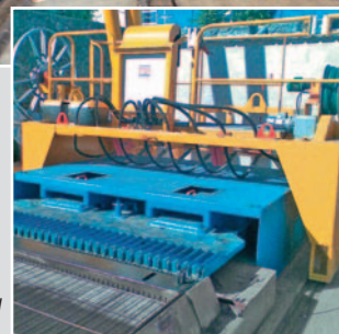
PRESLABS. Slipforming process.
