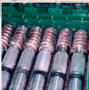
HOLLOW CORE SLABS. High frequency dynamic compaction extruder technology.
