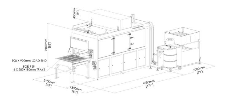
The Vapormatt Jaguar, compact and ergonomical, has been designed to fit in with state-of-the-art production facilities. It is constructed from high-grade stainless steel, continuously welded to form a water and dust-tight robust structure.
