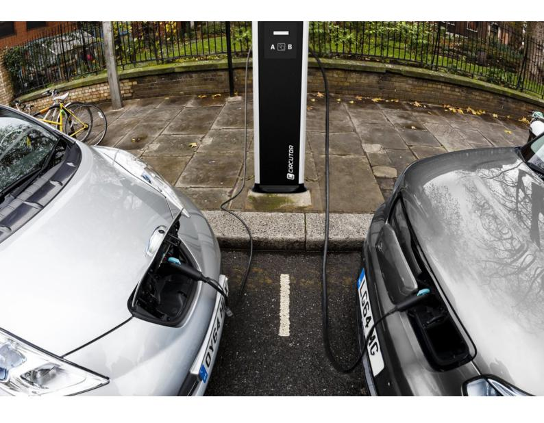
URBAN posts are designed for charging in outdoor car parks where the objective is both a robust and attractive unit. They have all the necessary electrical protection elements defined by the current standard for user safety.
