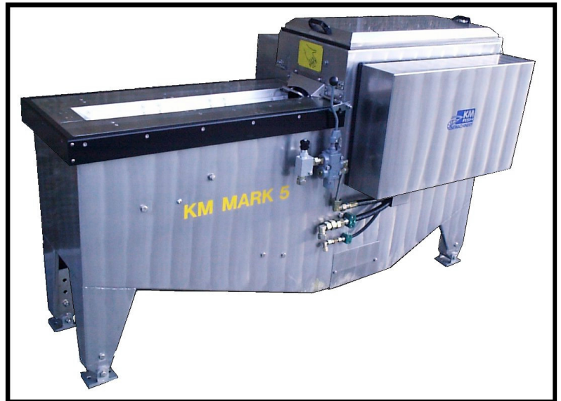
The KM. Mark 5 fish gutting machine for gutting cod, saithe, haddock whiting and hake.
