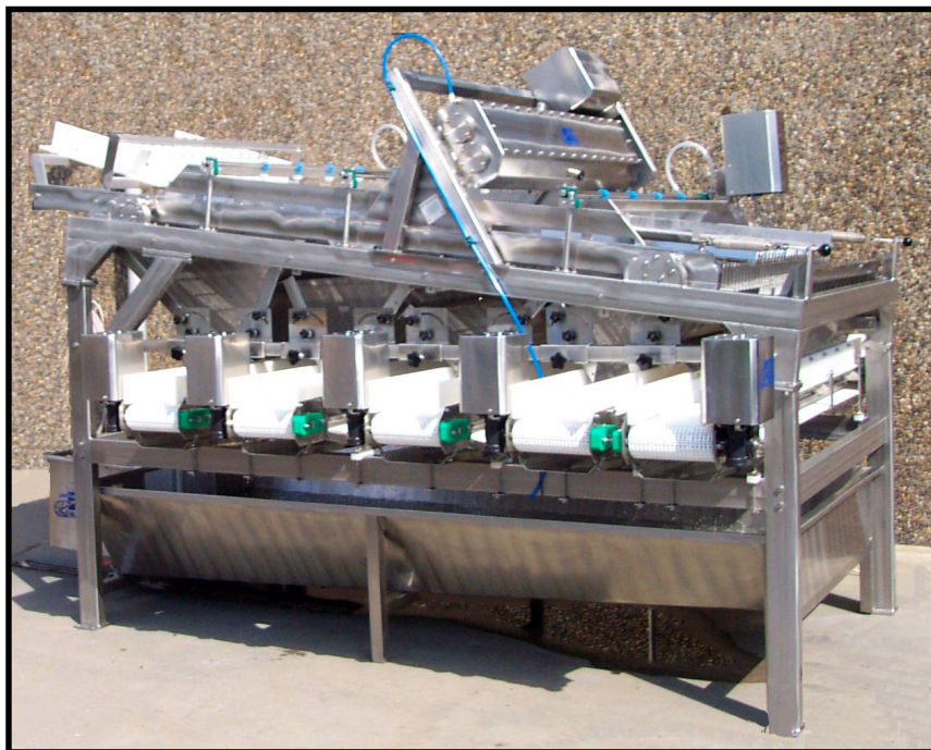
KM. 1400S Anchovy Grading Machine for grading anchovies before nobbing.
