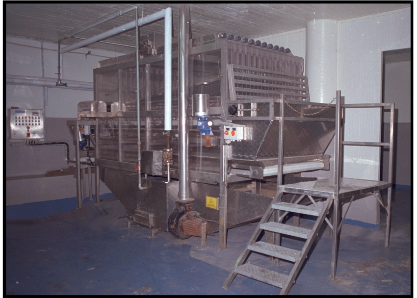
KM. 1200 Thawing unit for thawing block frozen and IQF frozen shrimp before grading and maturing.
