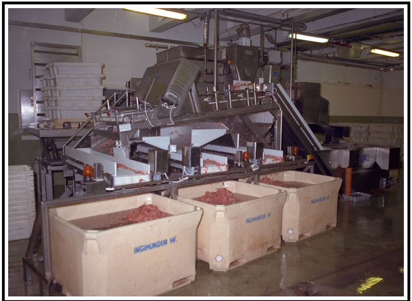
KM. 1140 Grading Machine for grading raw shrimp before being stored for maturing.
