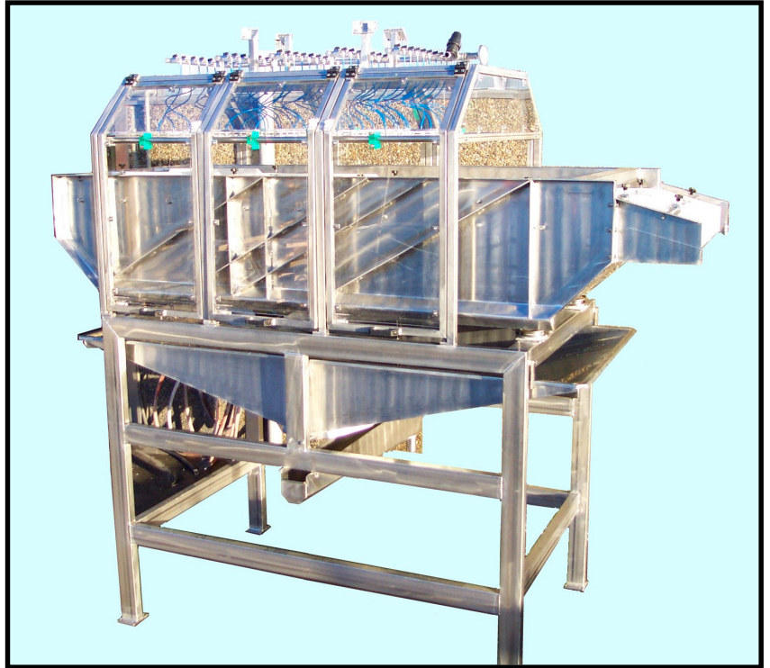
KM. 609/KM. 610 Glazing machine for glazing peeled, frozen shrimp.
