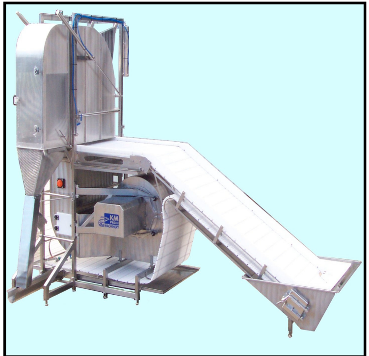
KM. 725 Air separator for separating shell from meat.
