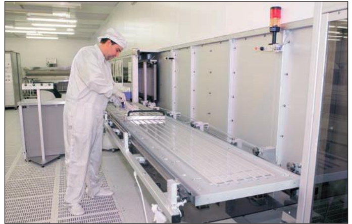
Vacuum machine for application of chromium layers
