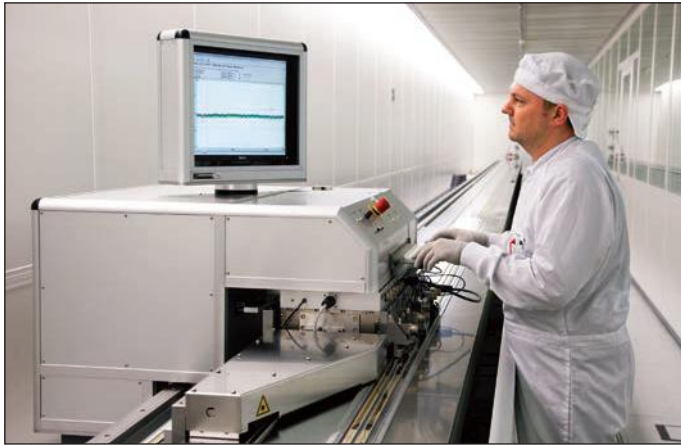
30 m long measuring machine for scale tapes
