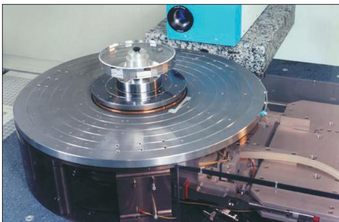
Angle comparator, measuring step approx. 0.001°
