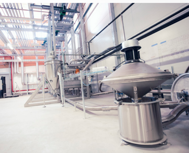
Left to right, top to bottom: chain hoist to lift the bags; ant dust filter; sifting system; multiline feeding
