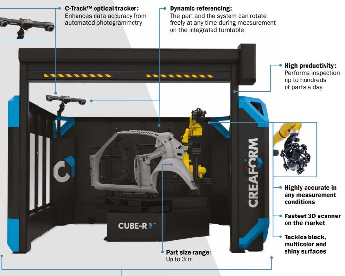
Complete turnkey solution: No integration required, fully enclosed and shop-floor-ready
