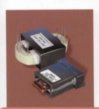
Planar windings have certain advantages over conventional winding systems. These advantages are mainly in size and effiency, with a typical efficiency of 98% being achieved, while their low profile makes them especially suitable for high density equipment designs. Other benefits of planar construction are very low leakage inductance, and minimum Electro Magnetic Interference (EMI).
