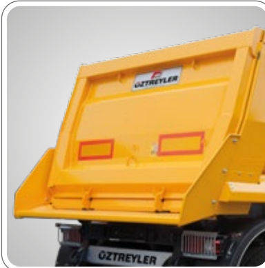
SPECIALLY DESIGNED AND REINFORCED MANUAL AND HYDRAULIC OPTIONAL REAR COVER
