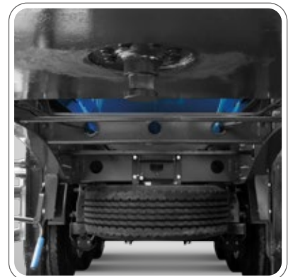
FLANGE KING-PIN REMOVABLE BY 2" BOLTS
