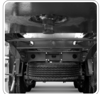
FLANGE KING-PIN REMOVABLE BY 2" BOLTS
