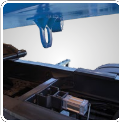
LOCK SYSTEM PREVENTING TIPPING WHILE MOVING BASED ON ROAD REGULATIONS
