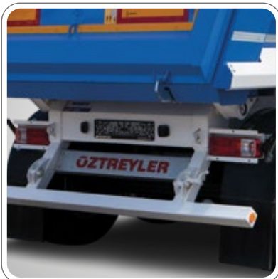
FIXED TYPE BUMPER (SAND AND EXCAVATION) FOLDING TYPE BUMPER (ASPHALT DUMPING)
