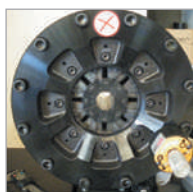
Large die opening = no need to remove dies Radial die travel = easy positioning of fitting
