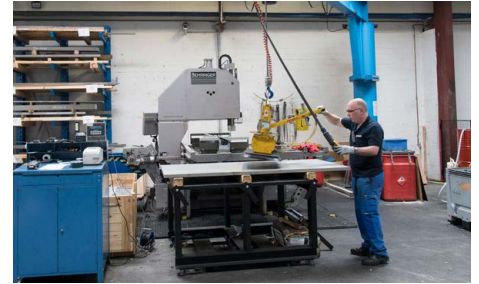
Kranbeschickung zu Säge Crane feeding to saw
