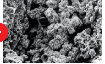
The size of the lead sulfate crystals is decreased, and the crystals are pitted as they are destroyed.
