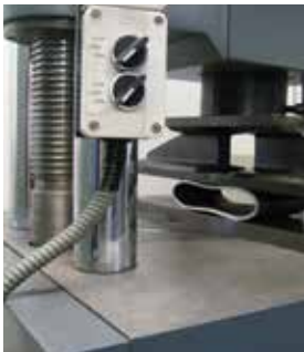
Yassılma Testi / Flatting Test TS EN ISO 8492 / ASTM A999 / ASTM A370
