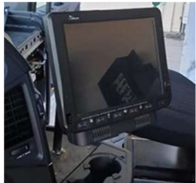
FM10Q VMC installed firmly on the truck
