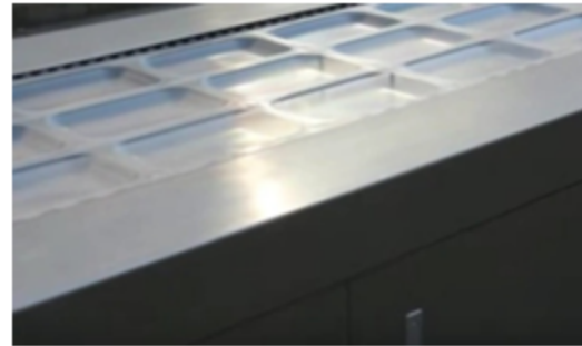
Forming of the bottom film
