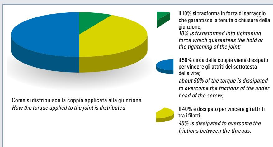
**COPPIA INDICATIVA DI SERRAGGIO (Nm / lb) IN FUNZIONE DELLA VITE | INDICATIVE TIGHTENING TORQUE (Nm / in lb) DEPENDING ON THE SCREW**
