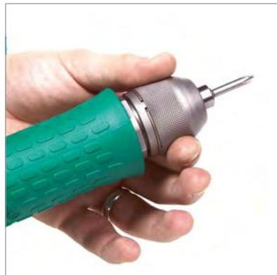
Adjust torque value rotating the external, milled ring nut.
