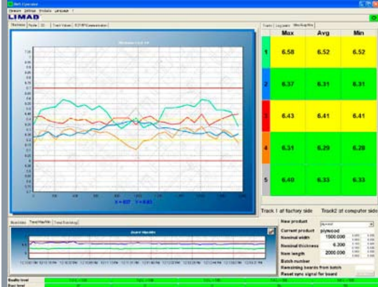
Operator display from a five track system showing thickness graphs, Max, Avg, Min values along with trend charts.
