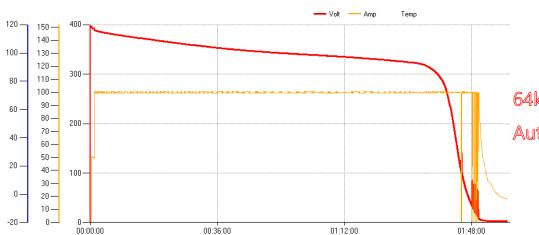
64kWh battery can be discharged within 2 hours. Auto short-circuit after discharge.
