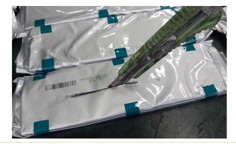
After short-circuit the battery, cell short cutting testing is perfect! (Better work process compare to salt water discharge)
