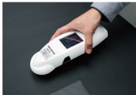
\Delta E , MI(Metamerism) management by spectrocolorimeter
