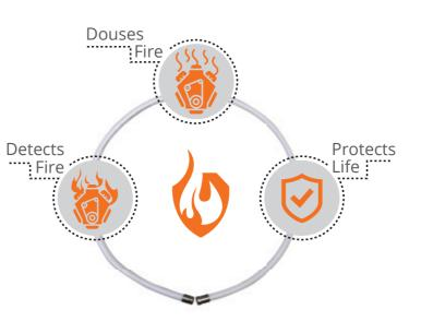
• Fits under the bonnet Senses heat during fire • At 120 degree Celsius, releases dousing agent • Extinguishes fire immediately.
