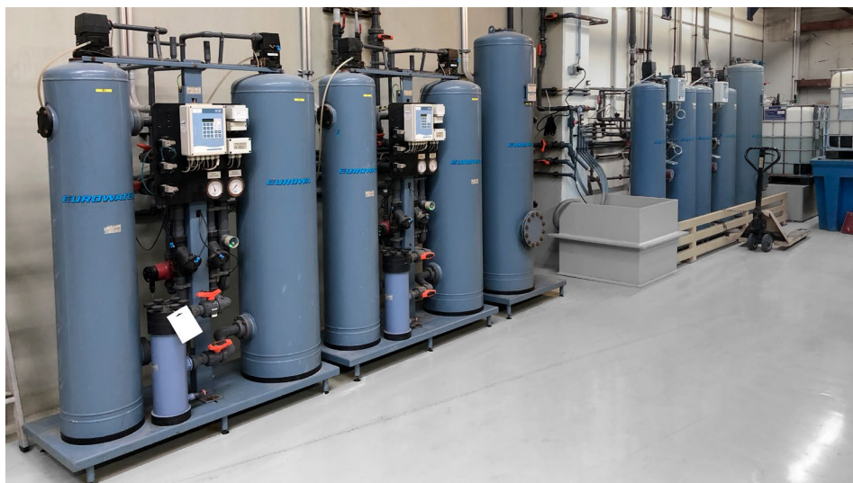
Multiple DI water production lines for pretreatment of light alloy wheels.
