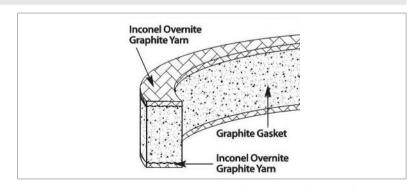
Increasing the contact area reduces the contact surface pressure of the inner fluid, and the circumferentially expanded gasket has a large airtightness due to strong surface contact, and the reinforced YARN can effectively suppress the extrusion phenomenon.
