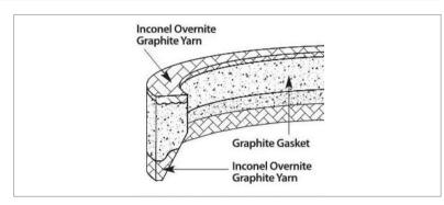
It is a bonnet gasket which is shaped like a valve bonnet. It is tightened by bolts and the bottom part is tightly tightened by strong compressive force. The reinforced yarn prevents CRUSH phenomenon against impact pressure.
