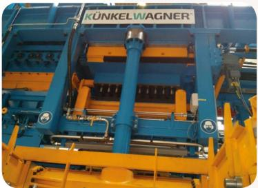
Kunkel Wagner moulding allows us to automate the production of larger castings that are outside the capabilities of our Disamatic lines.
