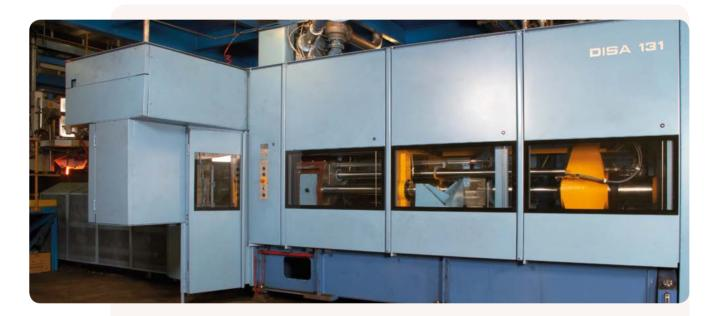
Our Disamatic 2110 and 131Z lines were installed in 2010 and 2012 respectively and together, allow up to 750 moulds per hour to be manufactured.
