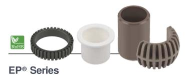
The EP® Series of engineered plastics bearings provide low friction and excellent wear resistance in many applications. Made of a variety of engineered resins compounded with reinforcing fibers and oil lubricant, they exhibit excellent dimensional stability, high compressive strength and creep resistance, low thermal expansion and good thermal conductivity.
