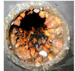
Bio-fouling Attachment of organisms (Bacteria and oysters attached to the pipe in the water)
