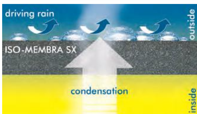
Performance principle of membrane seal
