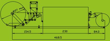
The **RG-200** is specially designed to manufacture pharmaceutical leaflets, allowing the incorporation of additional information, without changing the size of the leaflets. This is thanks to the integration of more sheets distributed at the same time, laterally joined by a small portion of glue.
