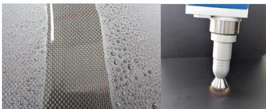
CFRP surface treatment before bonding and painting
