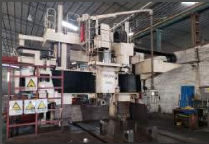
OKUMA GANTRY MACHINING CENTER Model No: MCM25x50E Specification: 5m*2.7m*2m Supplier: OKUMA
