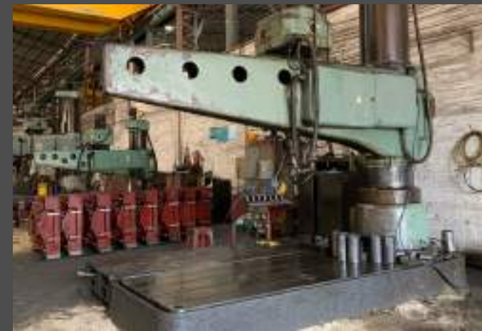
80 RADIAL DRILLING MACHINE Model No: Z3080×2.5 Specification: Max dia: 80mm height: 1800mm span: 2500mm Supplier: Zhongjie Radial Drilling Machine Factory
