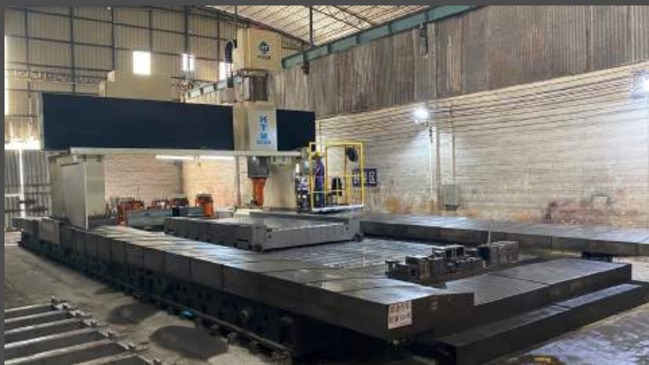
13 METER GANTRY MACHINING CENTER Specification: 13m*5m*2.1m
