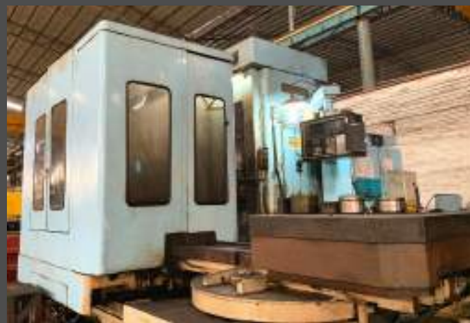
SHIBAURA HORIZONTAL MACHINING CENTER Model No: BMC-10B Specification: 1.2m*1.2m*1m Supplier: SHIBAURA
