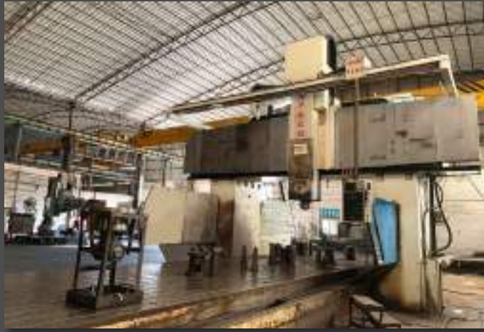
14 METER GANTRY MACHINING CENTER Model No: CPN30140T Specification: 14m*3.5m*1.6m Supplier: Weihai Huadong Automation Co., Ltd
