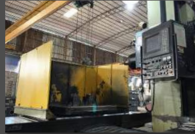
110 TOSHIBA HORIZONTAL MACHINING CENTER Model No: BTD-110R16 Specification: 2m*1.5m*1.5m Supplier: TOSHIBAMACHINE Co., Ltd
