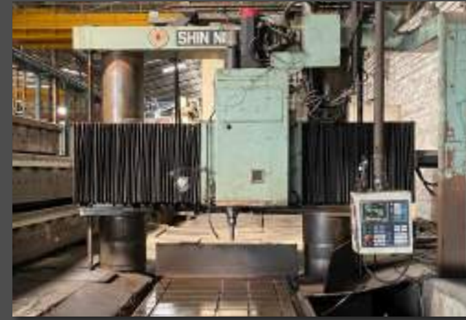
3 METER GANTRY MACHINING CENTER Specification: 3m*1.2m*0.7m Supplier: SHIN NIPPON KOKI
