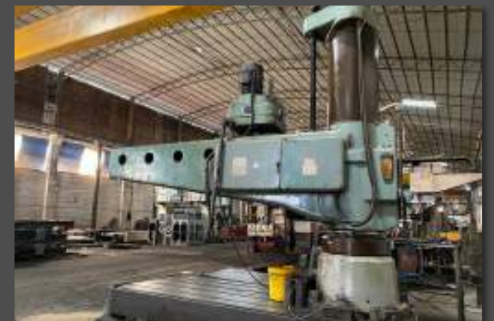
80 RADIAL DRILLING MACHINE Model No: Z3080×2.5 Specification: Max dia: 80mm height: 2200mm span: 2500mm Supplier: Zhongjie Radial Drilling Machine Factory
