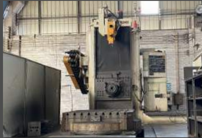
MITSUBISHI HORIZONTAL MACHINING CENTER Model No: M-HS125-NC Specification: 1.5m*1.5m*1m Supplier: Mitsubishi Heavy Industries Co., Ltd
