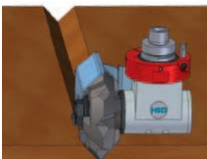
1 outlet for "Folding" ("V" grooving)
