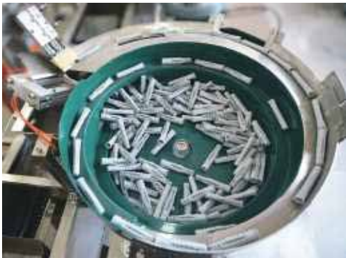
The standard materials are compatible, special material for special vibration plate 标准物料可兼容, 特殊物料专盘专用
