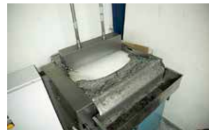
Hydrostatic band filter for filtering particles and metal chips from the coolant.
