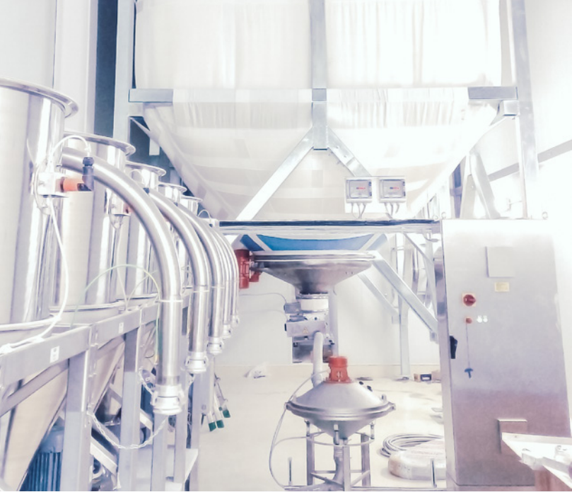
Silssystem with microingredient station, vibrosifter in pneumatic line and weight control; Silsystem group
