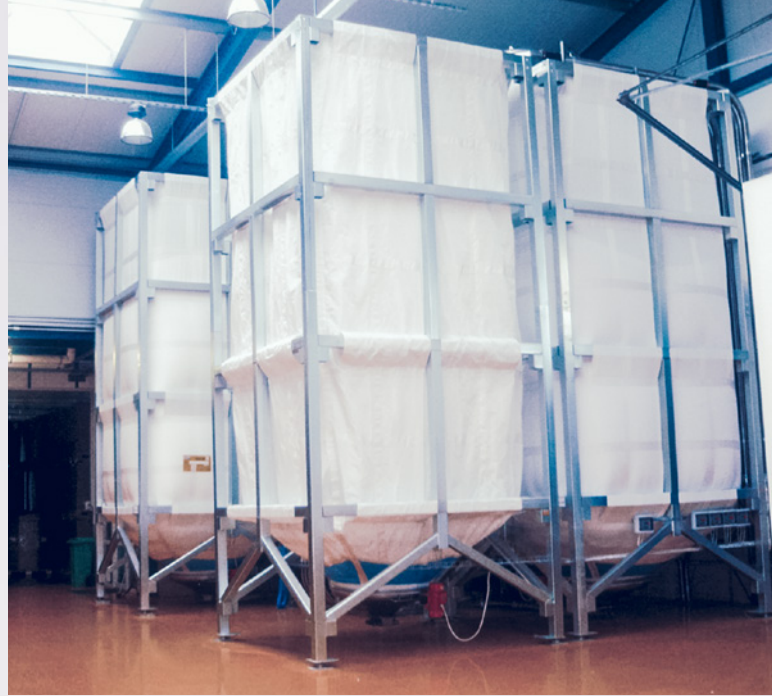
Silssystem with microingredient station, vibrosifter in pneumatic line and weight control; Silsystem group
