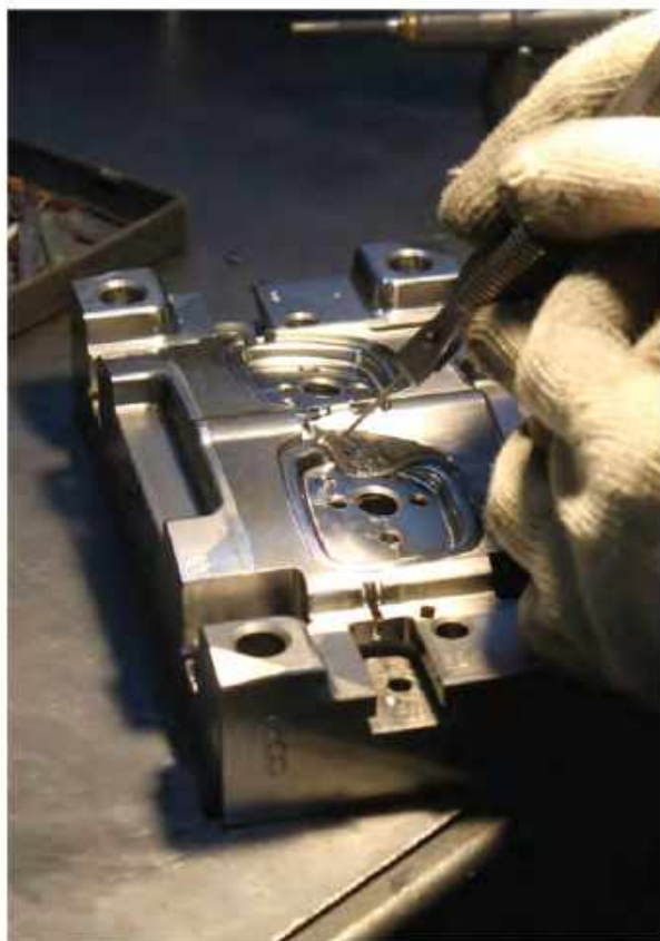
* Stavax | The stainless die steel with chromium alloy. Good corrosion resistant and wear resistance. The best material for the mold of plastic frames.
