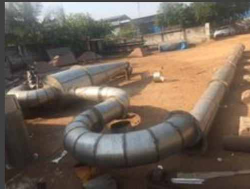
The principle of a flash dryer is simple. hot air (180oC) is sucked and mixed with the Wet product inside a very long pipe (called the flash pipe. The Wet product is passing through the pipe very quickly (in a "flash") and is dried to about 10% moisture.
