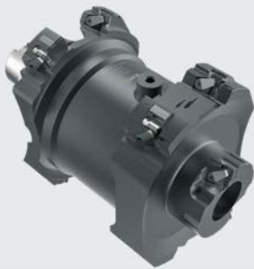
Fine boring tool with EA system with TEC indexable inserts Ø 70 / 185 mm, HSK-A63 - max. 11.5 kg
