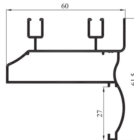
FN 600 DORMANT TUBULAIRE AVEC COUVRE JOINT
