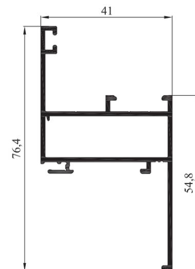
ATM 8017 DORMANT TUBULAIRE AVEC COUVRE JOINT
