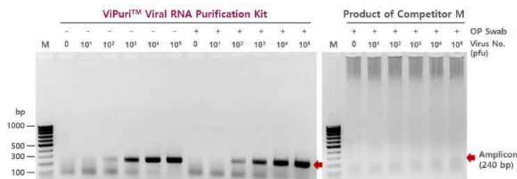
Fig. 2. Detection of the viral RNAs from an OP swab samples with mixed various amounts of +ssRNA virus (Norovirus) protected by rigid protein capsid. Single OP swab using Q-tip from healthy volunteers were dropped into 2 mL of PBS buffers with various virus particles. To isolate viral RNAs, 150 \mu L of the sample was processed with each kit then, 1 \mu L of final viral RNA elution was used for RT-PCR detection. The RT-PCR was performed using the One-step RT-PCR Master Mix with following conditions: reverse transcription at 50°C for 15 min; RT inactivation at 95°C for 2 min; 35 cycles of the following steps: 95°C for 15 sec, and 60°C for 30 sec.
