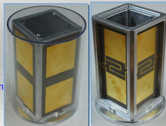
Omni-directional wrap-around antenna with CP (1x2 array, high gain)
