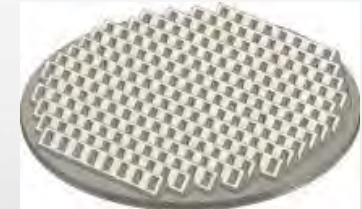
Circular Radiation Module with Tilted beam
