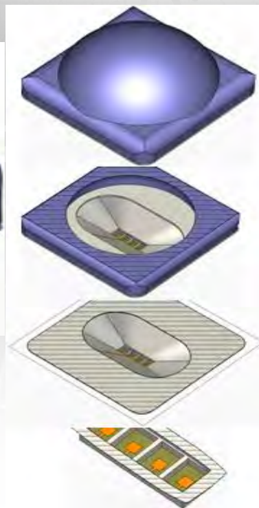
Lens antenna with 4-beams (integrated RF switching module)
