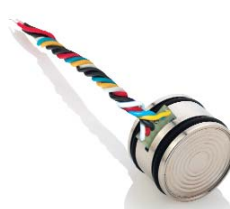
SERIE PD 9 L DIFFERENZ Ø 19 x 14 mm, nass/nass 0,1...50 bar diff. Basisdruck max. 200 bar
