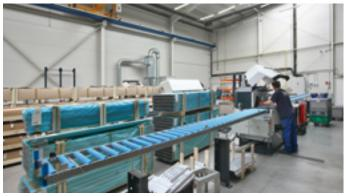
Usage of semi-automatic cutting machines for cutting of the main tubes of the trussing segments and a fully automatic machines for cutting of (the) main tubes of the tubes for bracing gives us an advantage of speed and precision.
