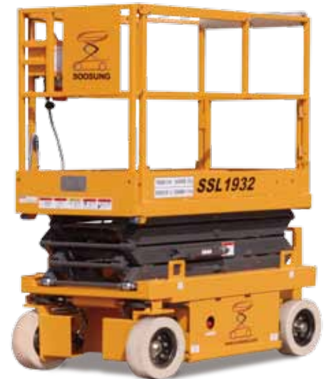
SSL-1932 ▶ Max. Platform Height 5.8M (Max. Working Height 7.8M)
