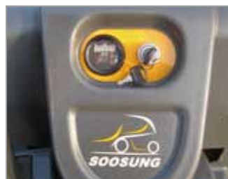
► Combined discharge indicator & Hour meter
