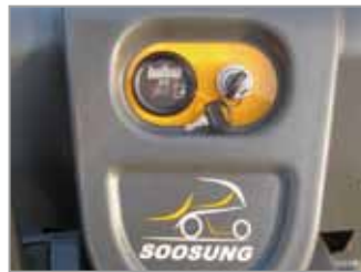
► Combined discharge indicator & Hour meter
