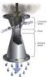
Capturing Gases through Spraying on Venturi
