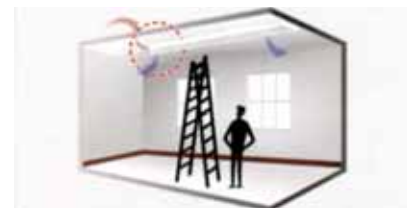
ceiling-installed type ERV Inconvenience for construction and maintenance
