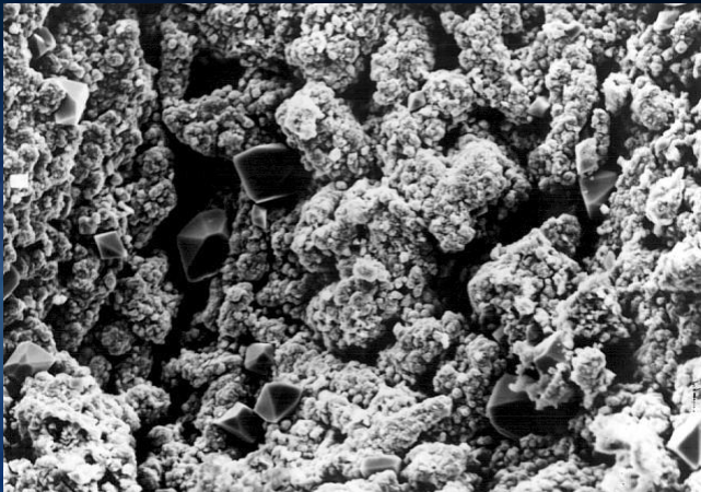
The final recovery of the plate to active sponge lead.
