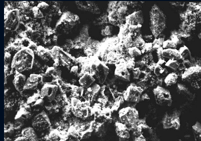
The size of the lead sulfate crystals is decreased, and the crystals are pitted as they are destroyed.
