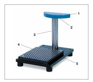
The base structure assembly is composed of bars, support feet, clamping devices, serrated referencing surface and support plate.
