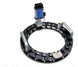
M4 Star ERG with lightened structure for extra large diameters
