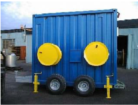
Fig..1 The wagon, control cabinet. Containing equipment for gas control and computer for temperature control
