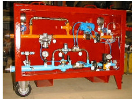
Fig.3. The Trolley. Gas and air trains
