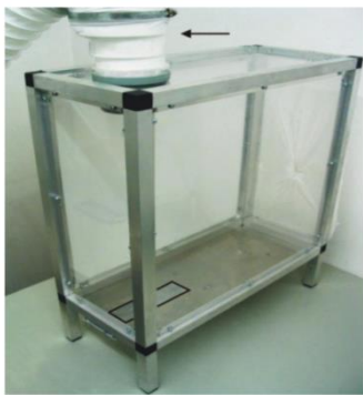
Fig. 1: BG Test Cage (front view). The air ventilation system is connected to the cage (black arrow). The arm is exposed at the test window in the metal floor sheet (black rectangle). The rear side is covered by gauze.
