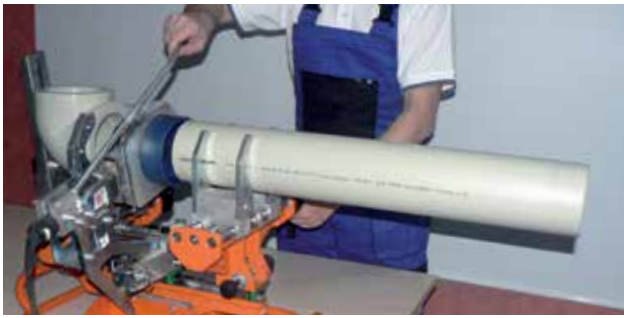
fixing and aligning the components, then heating them up
