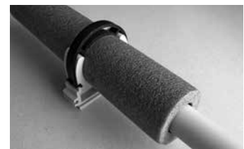
For hot water, the clip must be one size larger than the pipe (needs to be fitted over the insulation).
